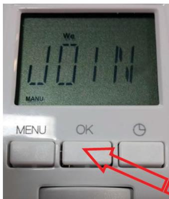
On the K470W valve will appear JOIN, then press OK
