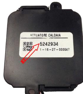
Enter the serial code on the A00850101 heater actuator and wait for device adding
